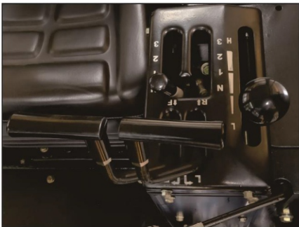
The operating mechanism is designed according to ergonomic principles, and the steering Joystick and throttle stick sideways to increase neutral Switching and reversing alarm for safer driving;
