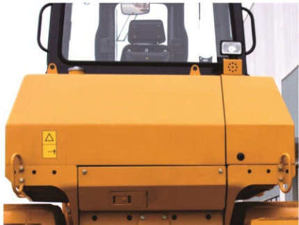
Use large-capacity fuel tank, the fuel tank volume reaches 580L, Continuous operation time is longer;
